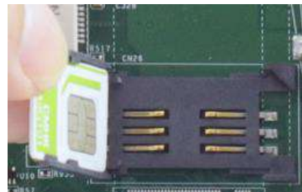
Insert Mini-SIM card with pins facing up
